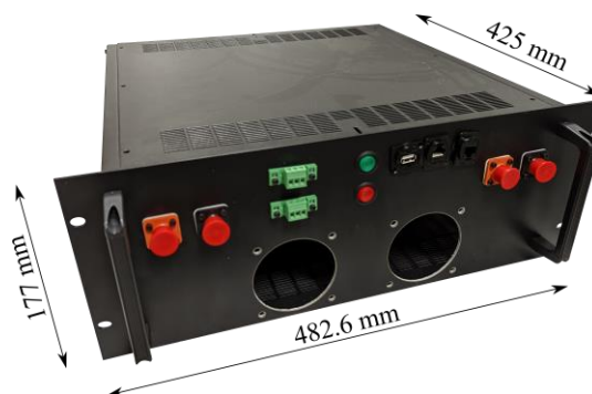
Fig. 6.14. Image of the assembled 19 inch rack.
