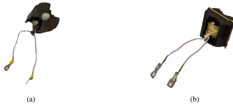
Fig. 3.7. Assembled inductances. (a) Single inductor case study ( L=150 \mu\text{H} and R_L=26 \text{ m}\Omega ). (b) Double inductor case study ( L=75 \mu\text{H} and R_L=31 \text{ m}\Omega ).
