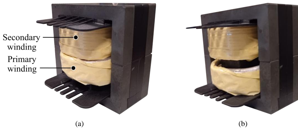
Fig. 6.16. Images of the assembled transformer. (a) Configuration for minimum leakage inductance. (b) Configuration for maximum leakage inductance.
