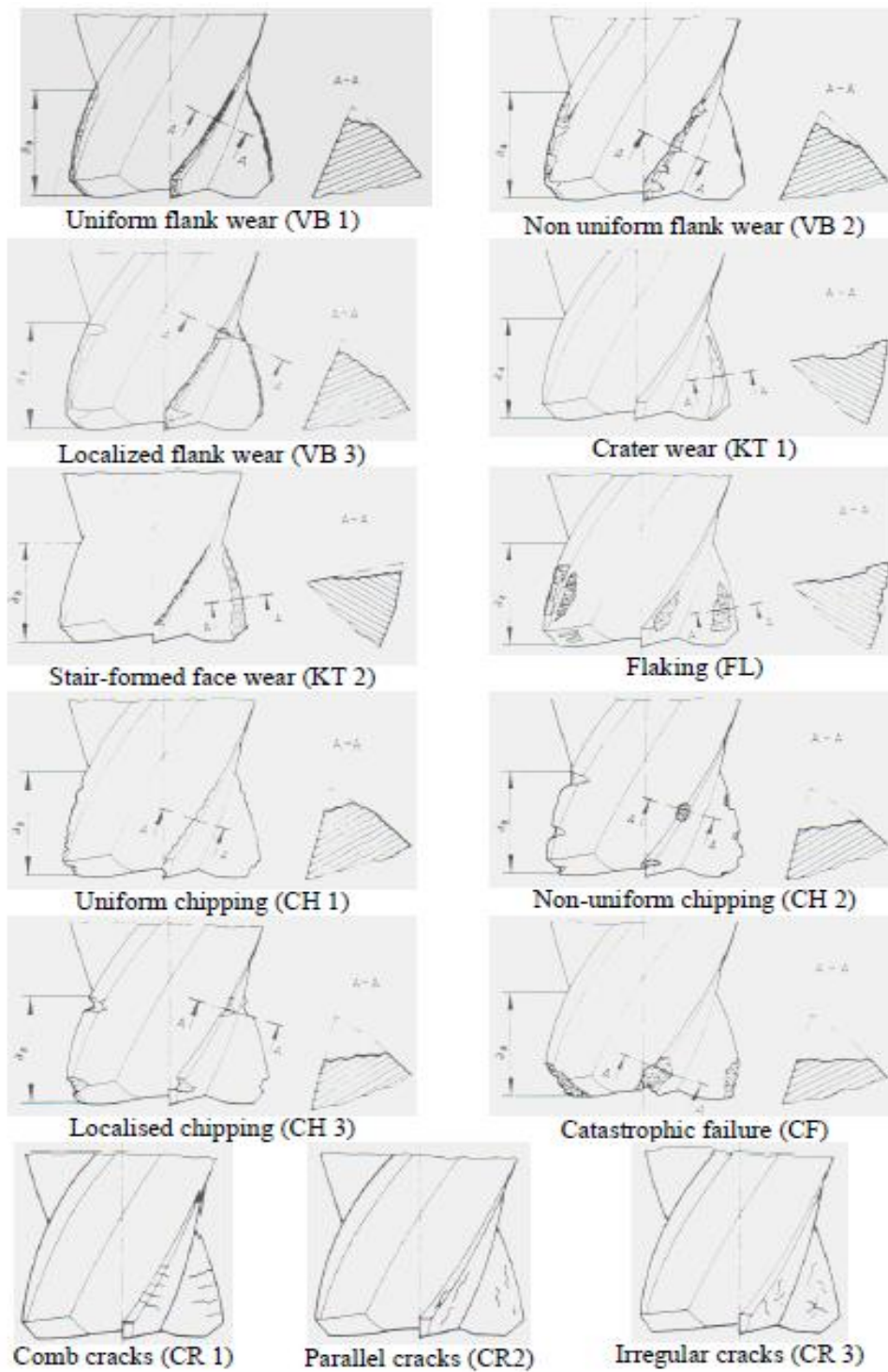
Figure 16 Tool wear types [84]
