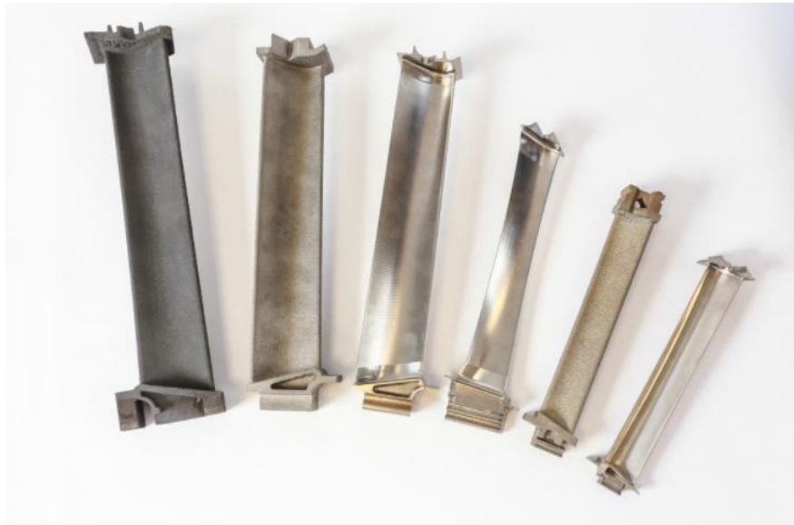
Figure 8 Additively manufactured GE blades in service [28]
