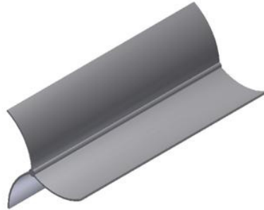
Fig. 2. The 3-bladed Savonius rotor geometry constructed for the numerical simulations
