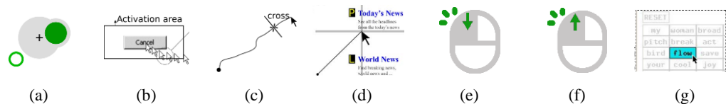
Fig. 4. Pictures of the adaptations suggested for problematic patterns: (a) bubble cursor, (b) magnetic target, (c) goal crossing, (d) cross cursor, (e) click on down, (f) click on up, (g) steady click.
