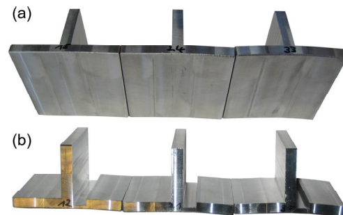
Figure 6: T-profiles applied with different loads, from left to right: F=35, 40, 45 kN, after bending (a) and after machining (b)
