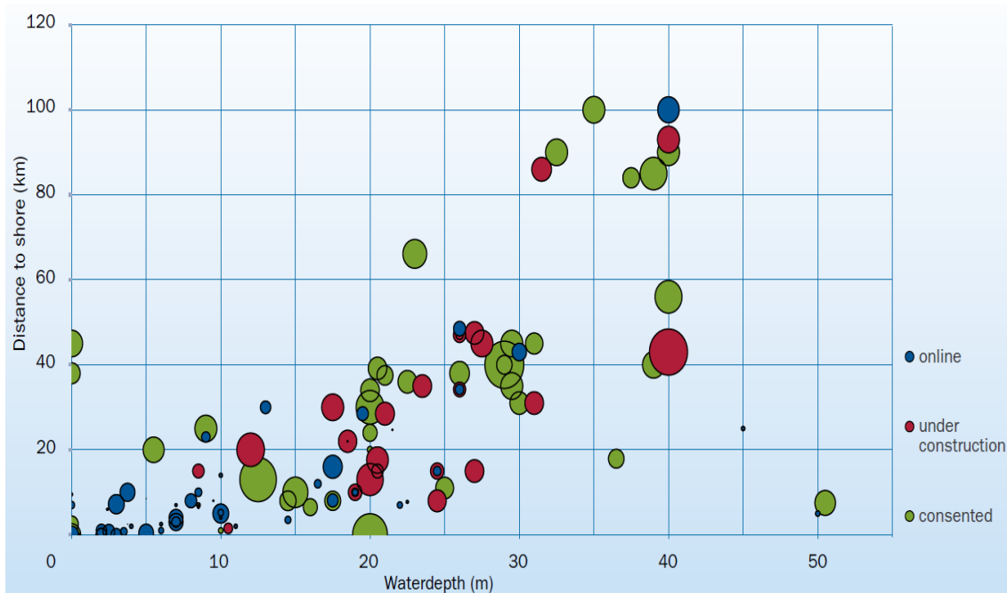
Fig. 1-5. Average size, distance to shore and water depth. Source: EWEA [2].
