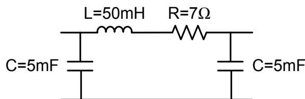
Fig. 1-16. Standard \Pi model using the parameters validated in [26] for a 100km line.
