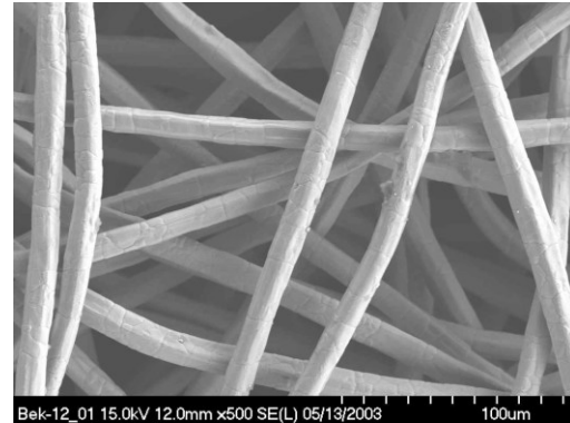
Figure 2. 16: Electron micrograph of a random fiber regenerator matrix. (Ibrahim, et al., 2007)
