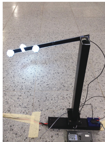
Figure A2. Setup of the reflective markers.
