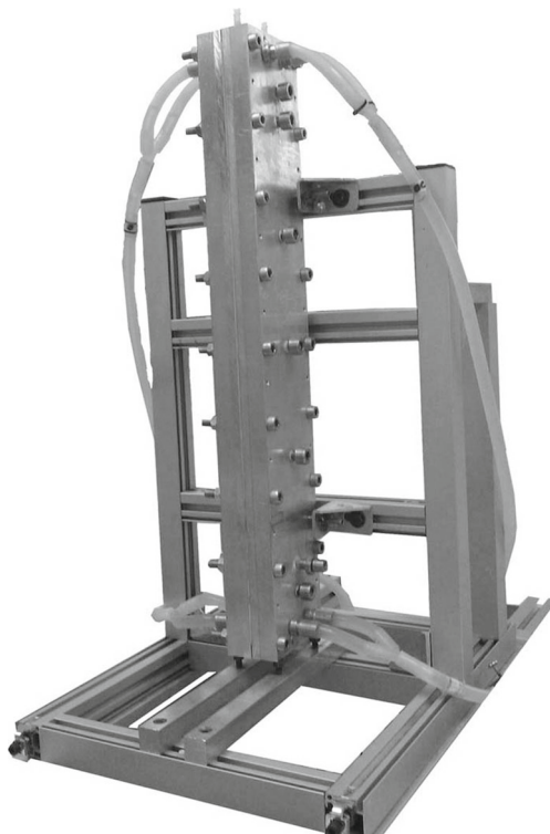
Fig. 1 Thermogravitational column with parallelepiped configuration
