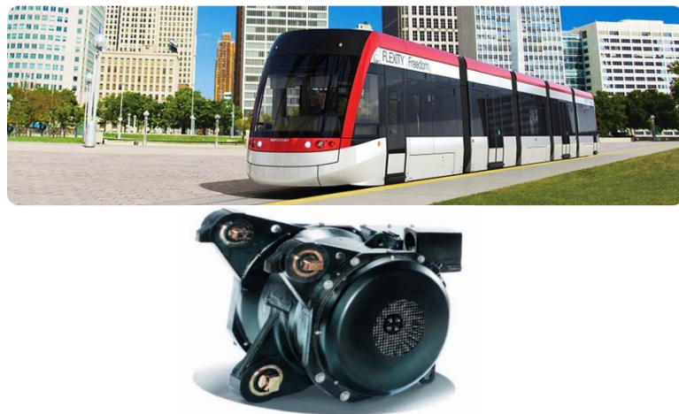
Figure 2.4. Bombardier MITRAC permanent magnet motor.
