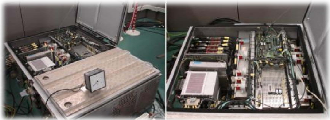
Figure 5.30. IGBT based inverter available in the laboratory.
