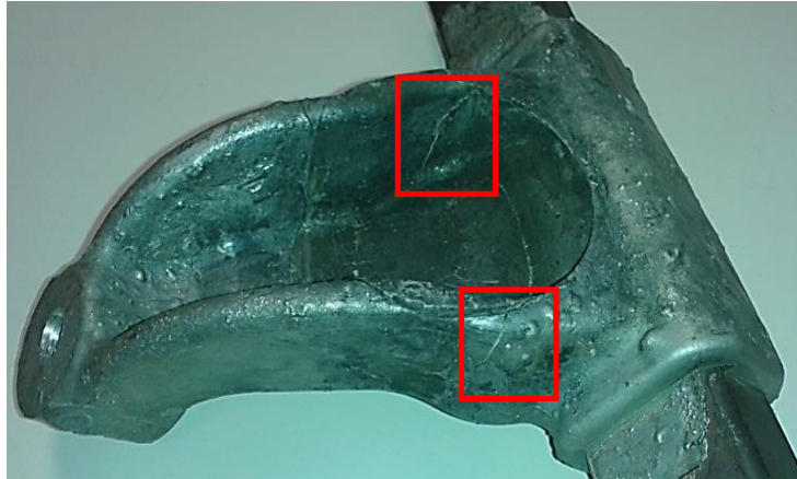
Figure 80. Early breakage of the component under fatigue.
