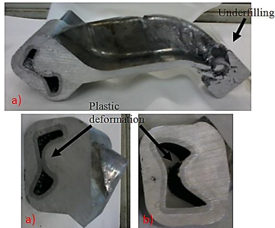
Figure 71. Details of cross sections of the body and the joint without bumpers.
