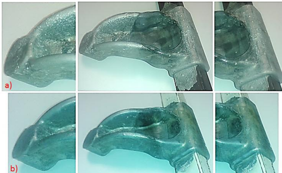
Figure 73. Hybrid structures after T6 heat treatment. Details of the head and the joining zone.
