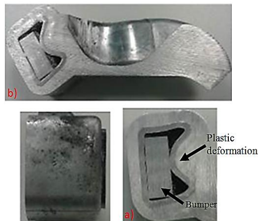
Figure 72. Details of cross sections of the body and the joint using bumpers.
