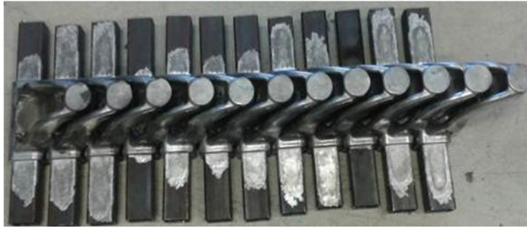
Figure 66. Batch of 12 hybrid components obtained by thixo lateral forging process.
