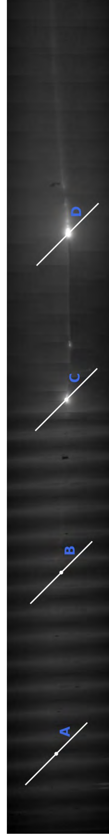
Fig. 4.10 Registered forged bolt with a delamination defect overlaid with profiles A and B in sound area corresponding to thread, C and D crack in flat area.
