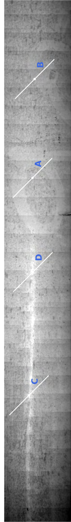
Fig. 4.25 Registered Steel billet with a delamination defect overlaid with profiles A and B in sound area, C and D crack.
