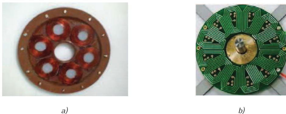
Figure 2-21: Coreless axial machines: a) coils flatten in resin [46] and b) PCB winding [53]
