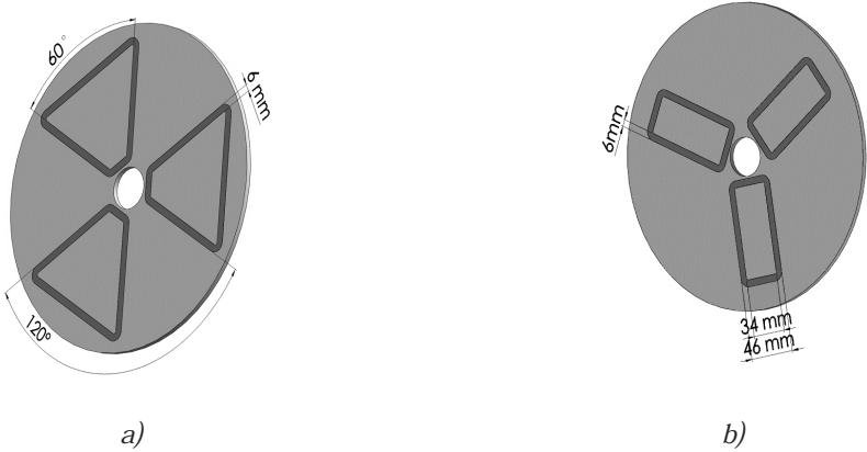
Figure 4-15: Views of the stators of the prototypes, a) trapezoidal coils and b) rectangular coils
