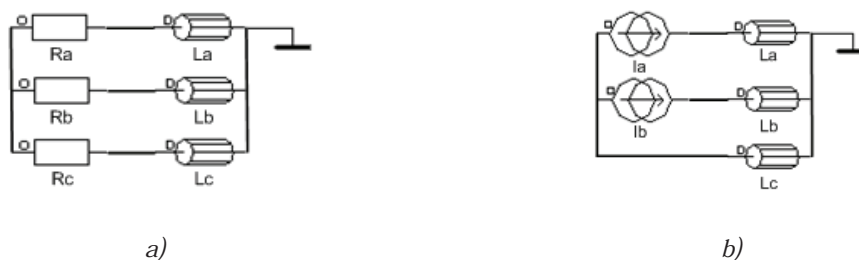
Figure 4-6: Coupled electrical circuits. a) open circuit and b) load circuit
