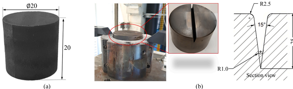
Fig. 1. a) T-shape test sample, b) (left) experimental grooved die, (right) the sectional view of the die.
