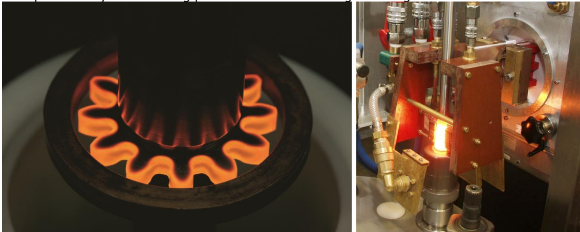
Figure 1. Examples of induction hardening of components. (a) A spur gear and (b) a shaft.
