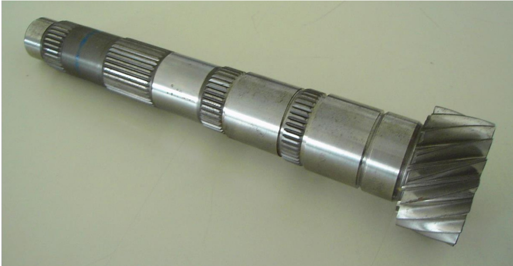
Figure 112. The secondary demonstrator, a secondary gear shaft in a Fiat manual gear box for a small car.
