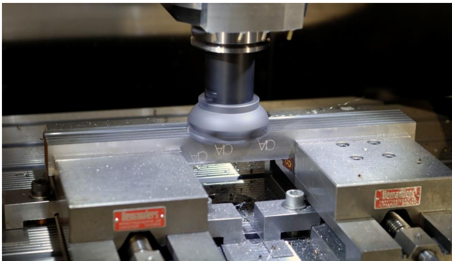
Figure 34. Configuration of the cutting tests. Face milling of bars made of the workpiece materials of the project.
