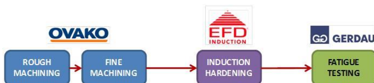
Figure 93. Manufacturing process for the QL-H1 (35CrMo4) and QH-H2 (50CrMo4) specimens fine machined before the induction hardening.
