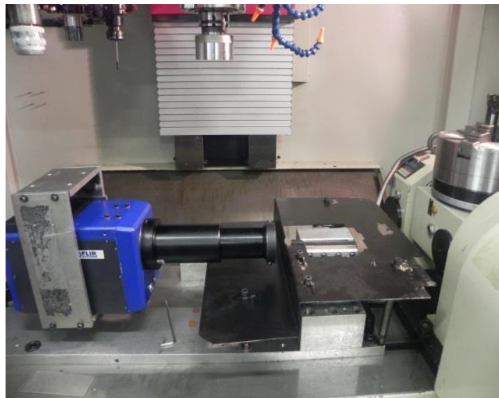
Figure 50. Experimental setup of fundamental cutting test in finishing turning.
