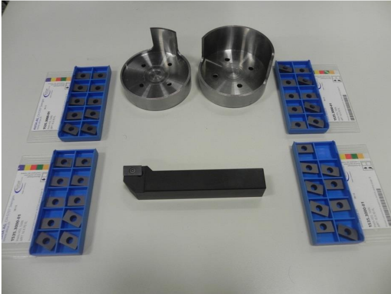
Figure 51. Workpiece specimen for interrupted orthogonal cutting in steel without heat treatment and cutting tool inserts.
