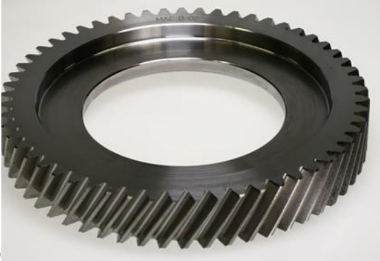
Figure 114. Soft machining of the demonstrator part. (a) As-forged, (b) turned and (c) gear hobbled.
