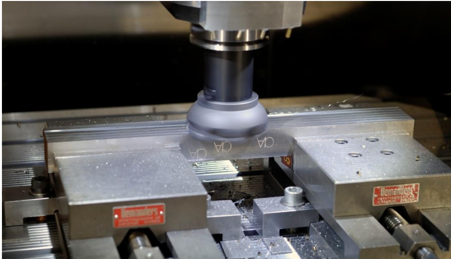
Figure 4. Configuration of the cutting tests. Face milling of bars made of the workpiece materials of the project.
