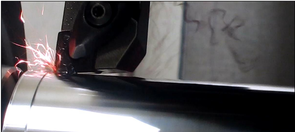
Figure 62. Photo from tool life test in hard part turning with CBN cutting tool in the Hardinge lathe.
