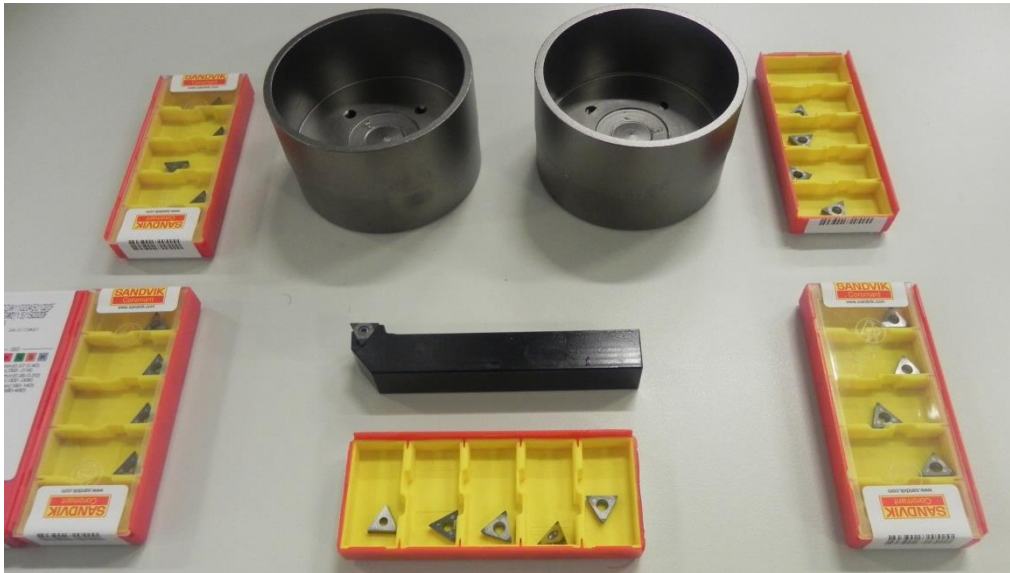
Figure 79. Workpiece specimen for continuous orthogonal cutting of hardened steels and cutting tool inserts.
