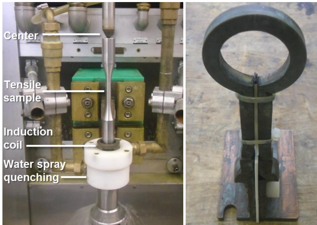
Figure 20. (a) Configuration of induction hardening of tensile test samples. (b) The induction coil.
