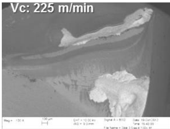
Figure 137. Micrographs of cutting edges used in tool life tests with 50CrMo4 (QH-T1). a_p=2 mm, f=0.4 mm/rev.
