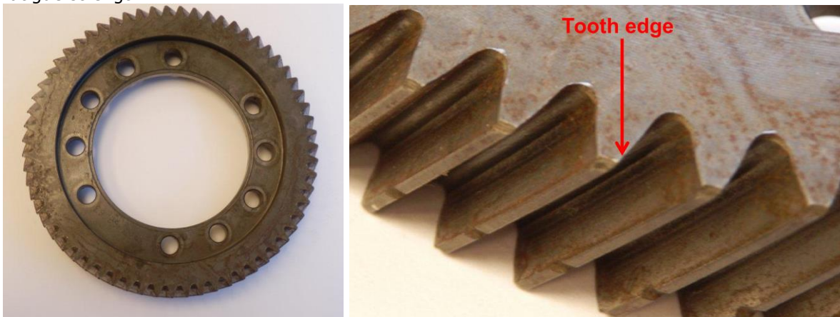
Figure 111. The primary demonstrator, a helical gear in a Fiat manual gear box for a small car.
