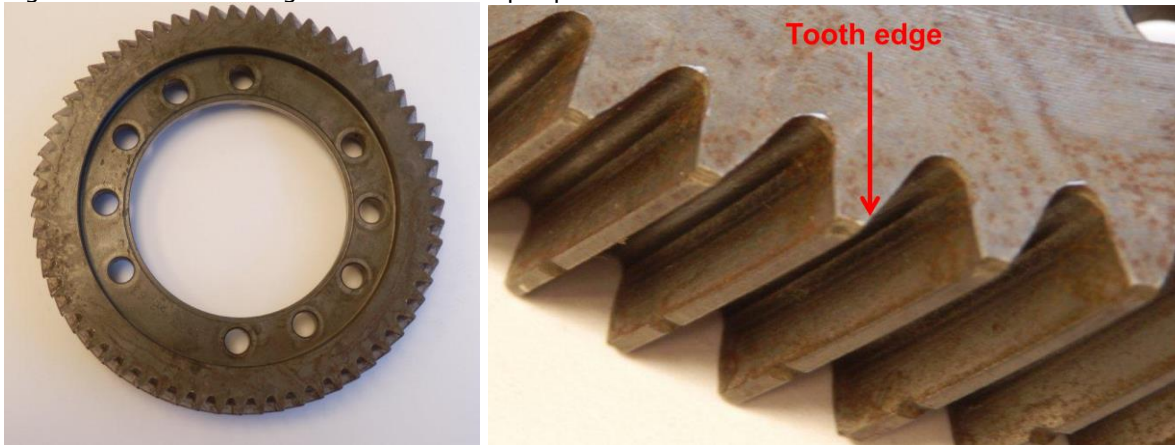
Figure 11. The primary demonstrator, a helical gear in a Fiat manual gear box for a small car.
