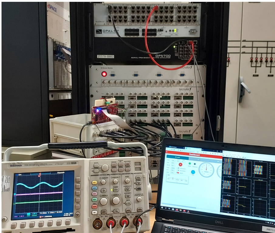
Figure 4.19: Opal-RT based real-time HIL testbed.
