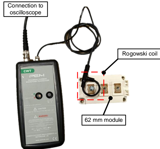
Figure 3. 21. Physical configuration of the current measurement on 62 mm modules.
