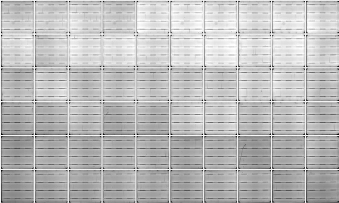
(b) Example of an Electroluminescence image of a solar panel.
