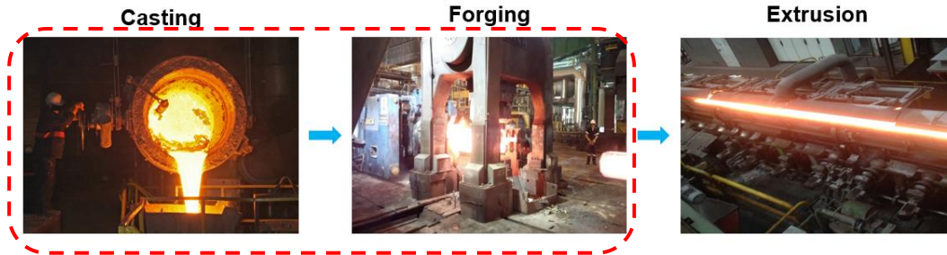
Figure 1-2. Seamless tube manufacturing process.
