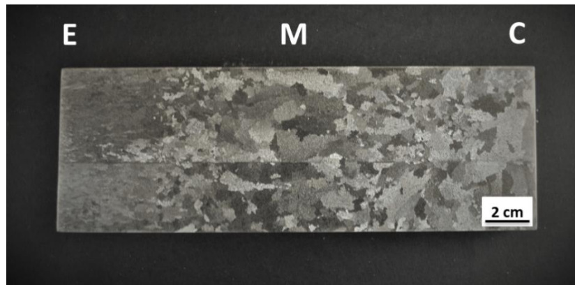
Figure 4-2. as-cast microstructural grain map for the Alloy 28.
