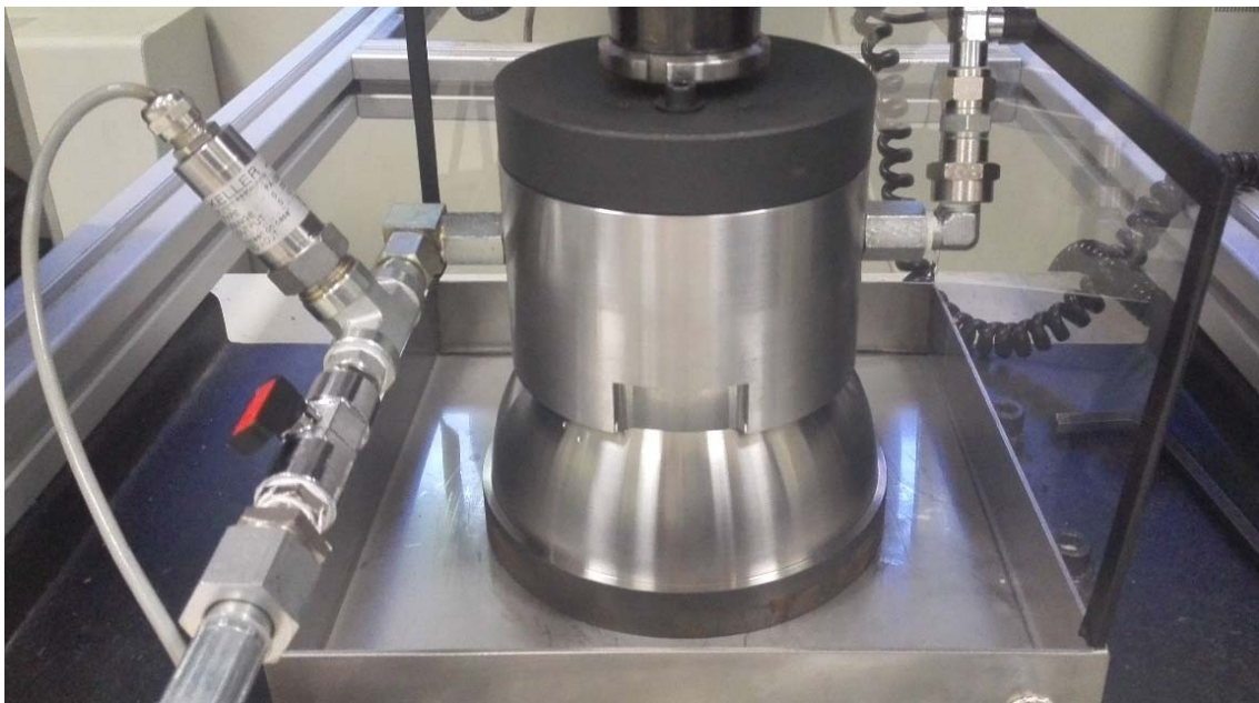
Figure 5.2: Slotted seat testbench in the universal testing machine.
