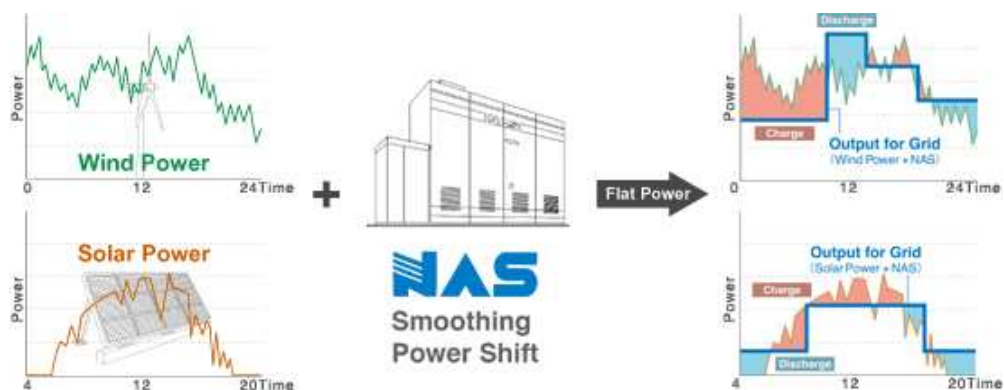
Figure 6: ESS to stabilize intermittent renewable energies. Source: NGK insulators.
