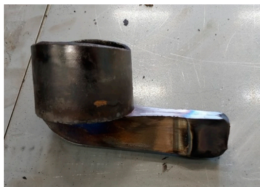
Figure 6. Obtained component after the first NSF trial with the 42CrMo4.
