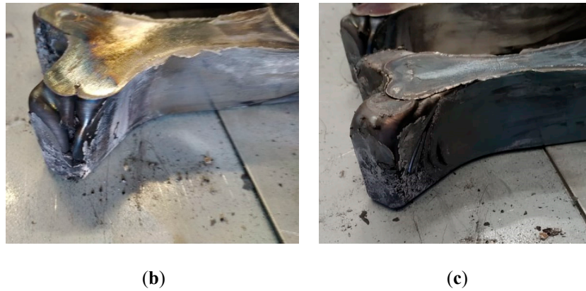
Figure 8. (a) Obtained components in Trials 1, 2 and 3, respectively, (from left to right). Detail of the last part filling (fingers) in (b) Trial 2 and (c) Trial 3.
