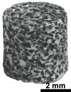
Figure 2.2: Scaffold with a porosity of 72-76 % with pore size of 10-1000 \mu\text{m} [Wit07a, Wit07b]
