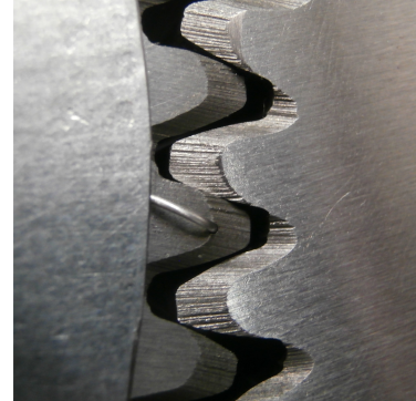
Figure 7.4: Thermocouple inserted in small module tooth
