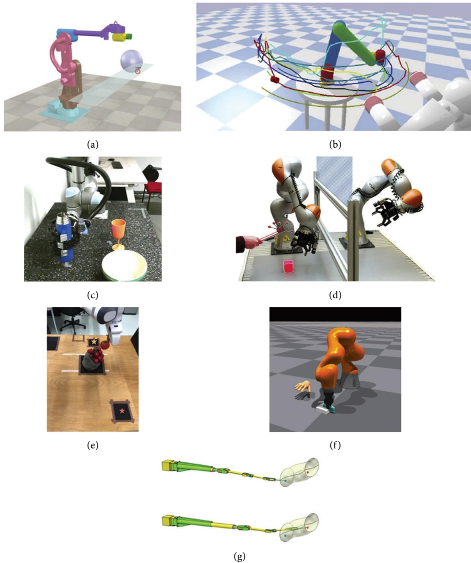
FIGURE 8: Motion planning evaluation scenarios: (a) and (b) via-point tasks [44, 51]; (c) pick-up tasks [90], (d) and (e) pick-and-place tasks [78, 89]; (f) disassembly tasks [94]; (g) duck-enter tasks [97].
