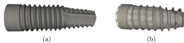
Figure 4.1: Images of the analyzed dental implants acquired by the ALICONA system with the 3D rotation unit. (a) BTI Tiny (BT) and (b) BIOMET 3iT3TM (BM).
