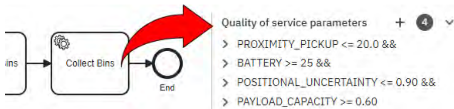
Figure 6.4: Defining quality conditions using the “AAS Web Service Discoverer” plugin for Camunda Modeler during the workflow design phase.
