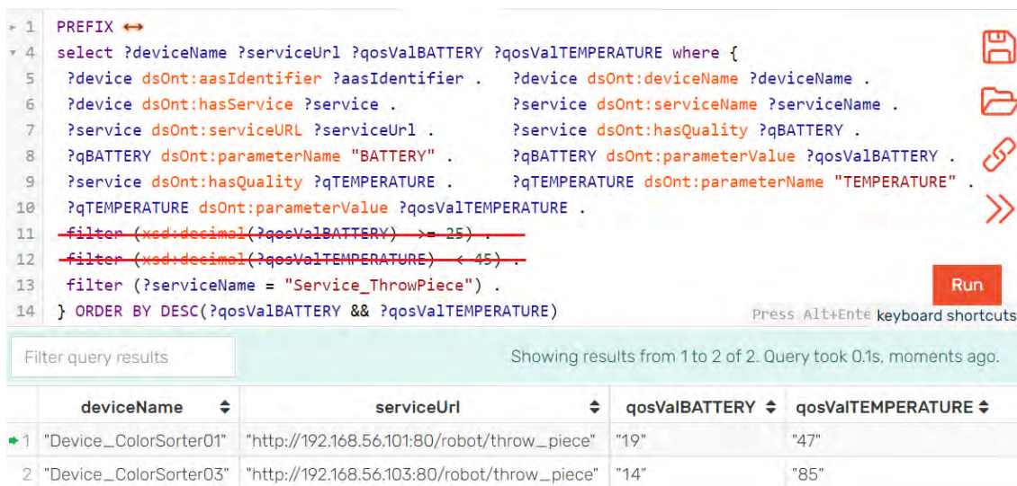
Figure 5.8: SPARQL query and results for case 4 “When none of the devices/services aligns with any quality condition”
