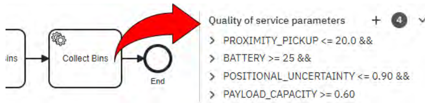
Figure 4.7: Defining quality conditions for a workflow task in Camunda Modeler and the AAS Service Discoverer plugin
