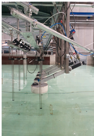
Fig. 2. Picture of the array of scaled Wavestar prototypes, together with a schematic representing the main components of a single device belonging to the considered arrays.
