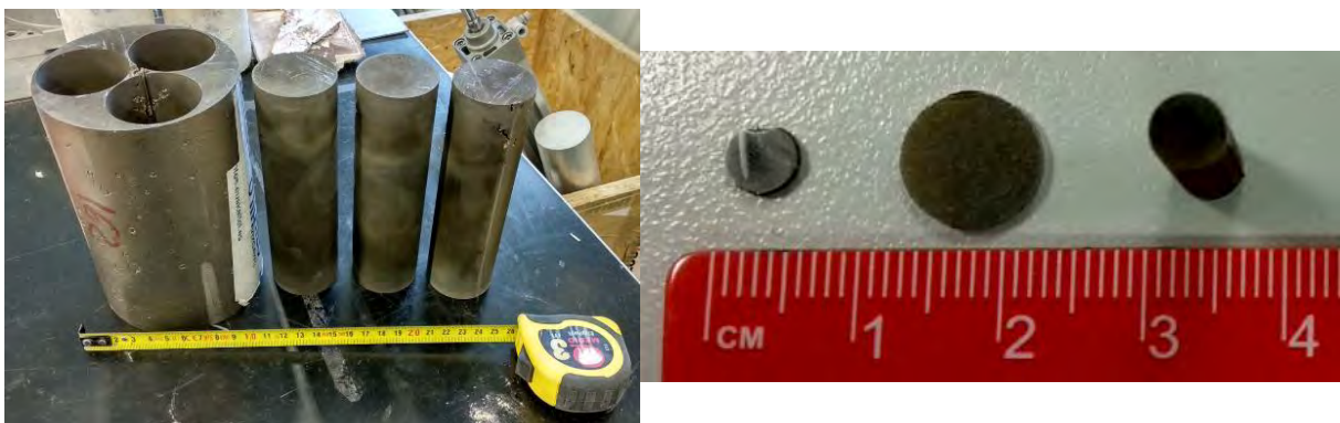
Figure 3-5. a) As-cast Inconel 718 superalloy ingot. b) Samples for thermal characterization.
