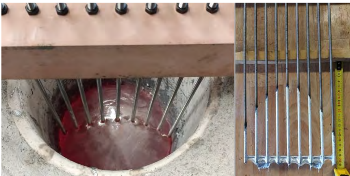
Figure 5-6. Experimental setup for free surface deformation measuring device.
