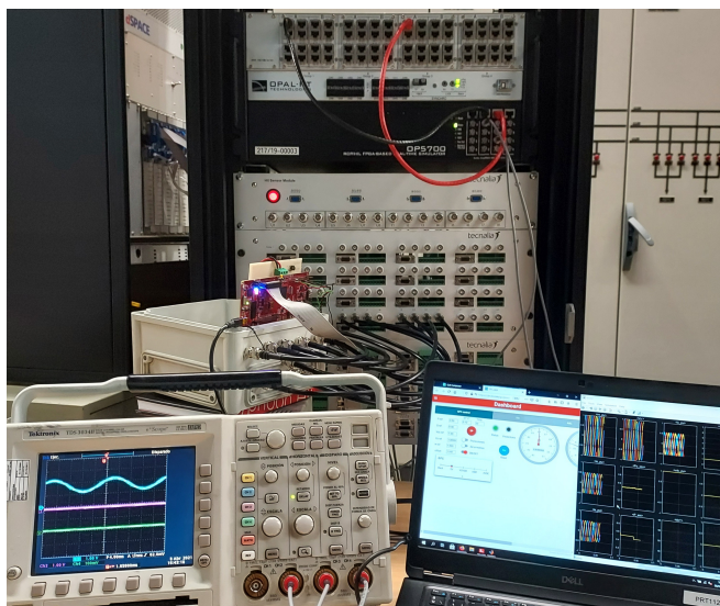
Fig. 15. Opal-RT based real-time HIL testbed.
