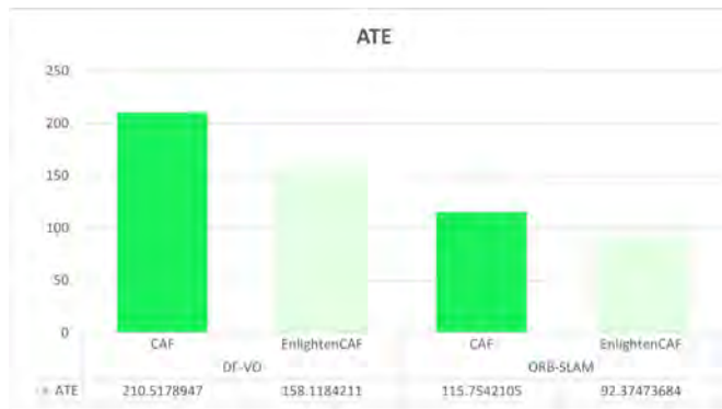
FIGURE 12: Comparative of ATE when applying DF-VO and ORB-SLAM2 algorithms in CAF and EnlightenCAF datasets.
