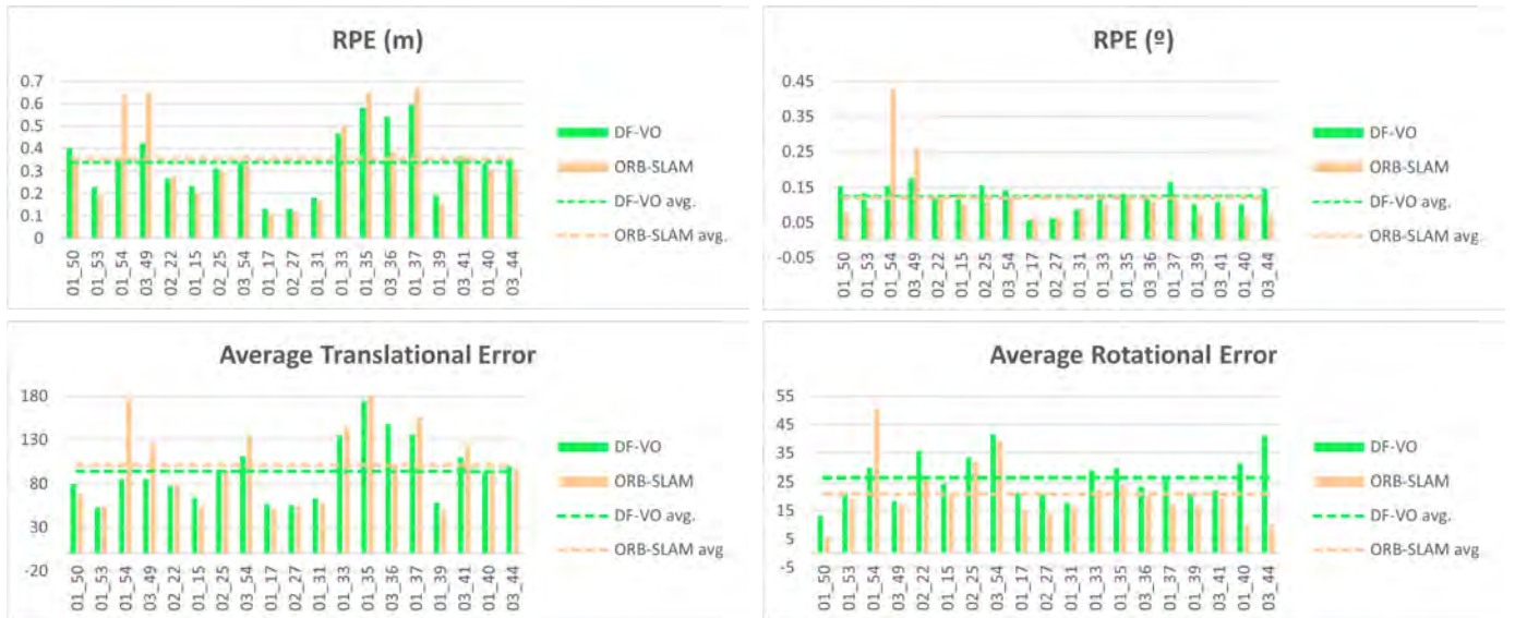
FIGURE 9: Comparison of relative VO evaluation metrics when applying DF-VO and ORB-SLAM2 algorithms in CAF datasets. Translational and rotational components of relative errors are shown separately.
