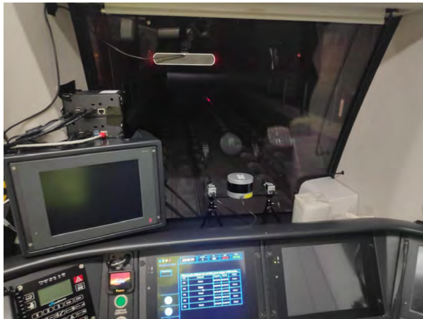
Figure 3.4.: Camera placement for CAF use case. Camera was placed in the front of a moving train in an urban underground railway scenario.
