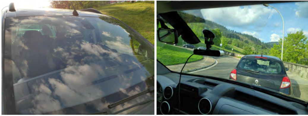
Figure 3.6.: Camera placements for CarDriving use case. The camera was placed in the top part of the windscreen of a car moving on an urban scenario.
