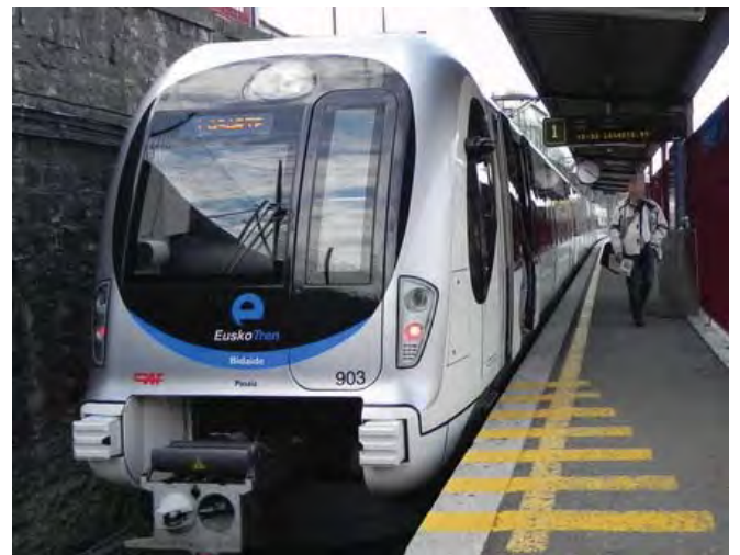
Fig. 1. Signaling patterns are placed at the end of the platforms, as the yellow pattern shown in this figure.
