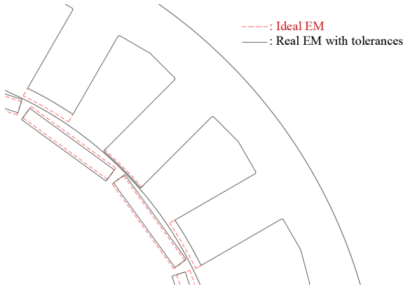
Fig. 2. Example of PMSM with rotor tolerances and stator tolerances
