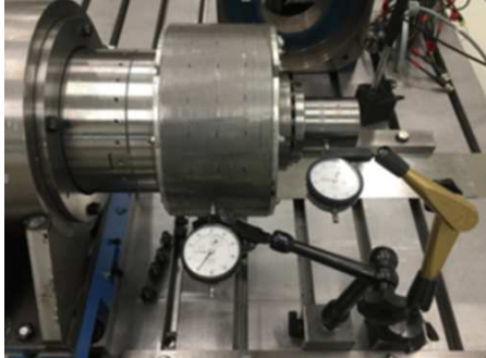
Fig. 7. Measurement of the poles of the rotor by means of dial indicators
