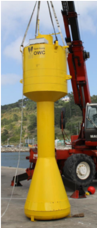
Fig. 1. 1:16 scale prototype of the Spar-buoy OWC is a floating oscillating water column [22].
