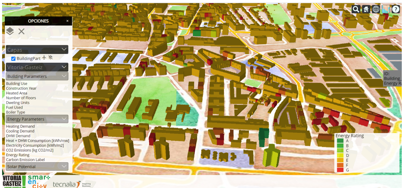
Figure 6. Dashboard for the GIS-based energy services for energy demand and usage visualisation.
