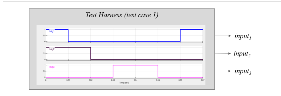
Figure 4.9: A harness block containing a test case. The test case is composed of three signals (input vectors). The fixed time step is set to 0.01sec , thus, each input vector provides 8 values during simulation.
