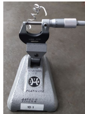
(b) Cut chip measurement V_c400fz0.2ap2 .
