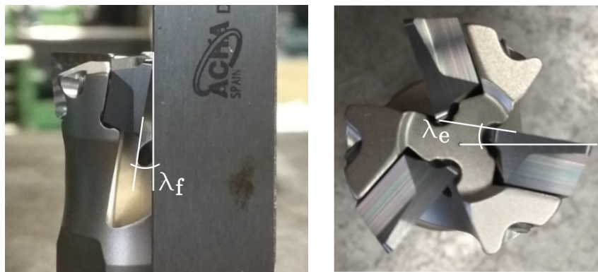
(a) Insert flank rotation angle 8^\circ .
