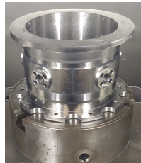
(b) Result of face milling 1202.
