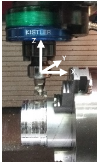
Figure 3.20: Orthogonal centric turn-milling experimental setup.
