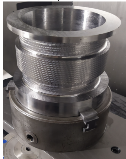
(f) Machining results of operation 2105 with depth of cut ( a_p = 2 mm).
