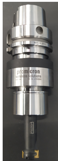
(a) Promicron Spike (R) and the flat end mill Sandvik (490)
