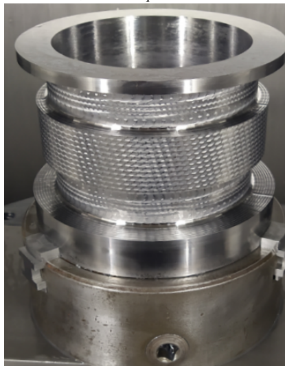
(e) Machining results of operation 2105 with depth of cut ( a_p = 1.25 mm).
