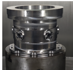
(a) second clamping event, internal diameter clamping.
