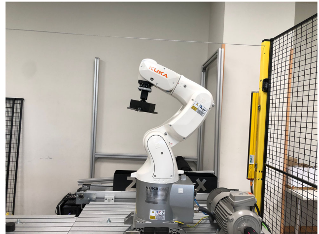
Fig. 5 The optimal standby pose obtained by minimizing the total torque applied by the joints with the multiobjective genetic algorithm
