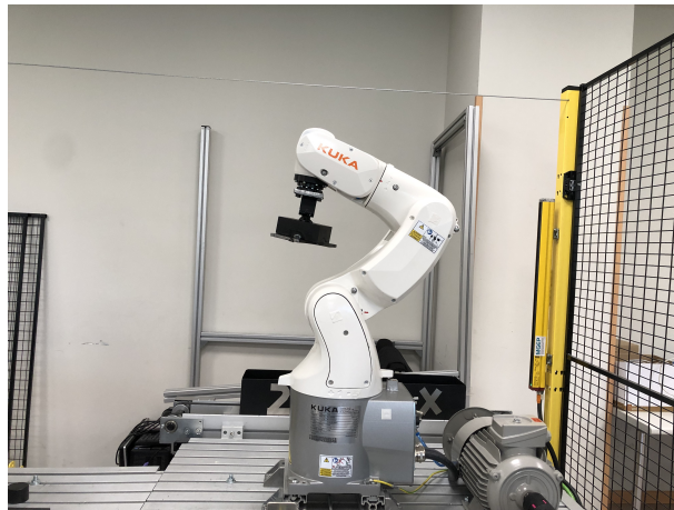
Figure 4.20: The optimal standby pose obtained by minimizing the total torque applied by the joints with the multi-objective genetic algorithm.
