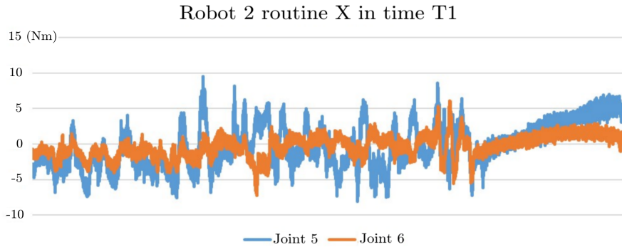
Figure 4.29: Synchronized data acquisition of Robot 2 (joints 5 and 6) executing routine X in time T1 .
