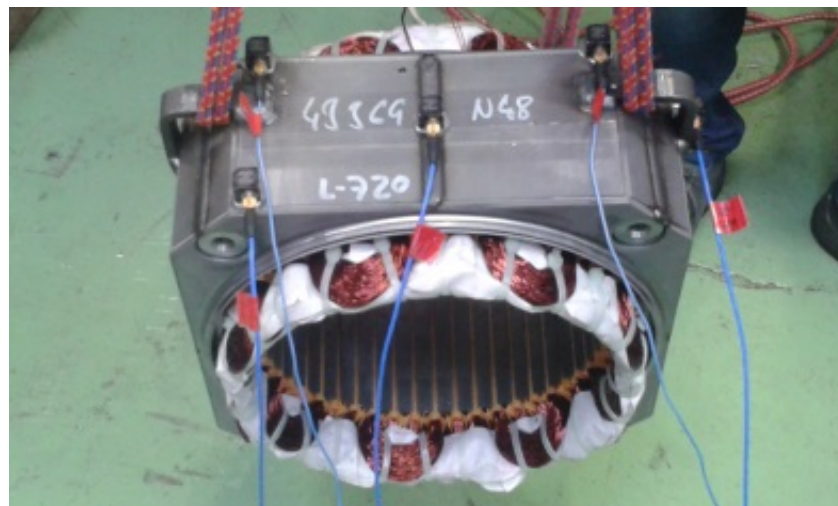
Figure 2. Experimental setup of the measurement of the natural frequencies of the stator.
