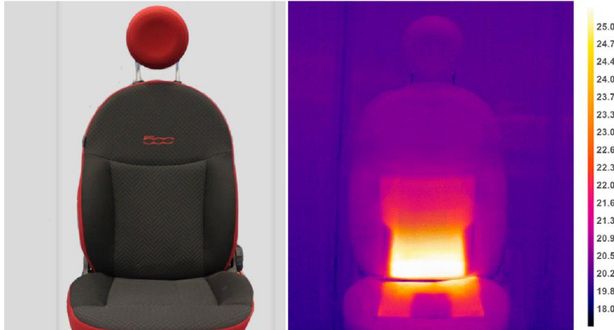
Fig. 7 Surface temperatures of the seat in heating operation
