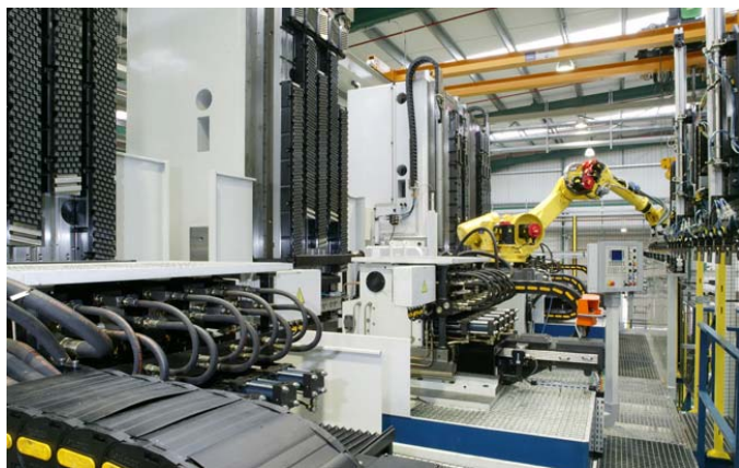
Figure 40. External broaching machine equipped with a robot [24].
