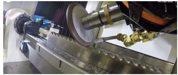
Figure 33. Final grinding of a broaching tool [90].
