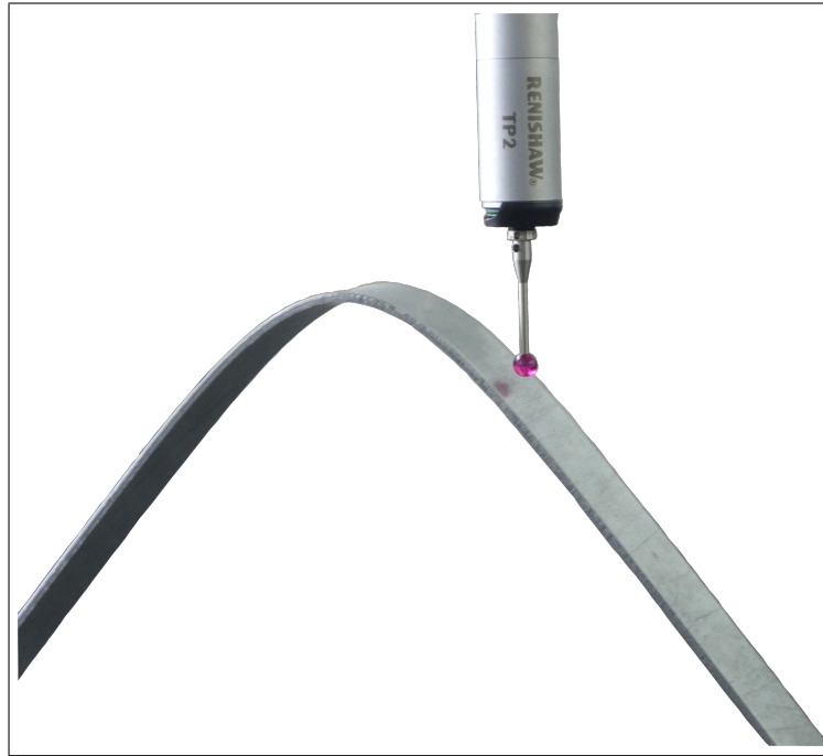
Figure 6.2. Sample measurement using a 3D coordinate measuring machine Mititoyo BHN710.
