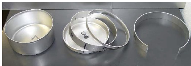
Figure 2.13. Demeri cup, split-ring test, experimental procedure (Laurent et al., 2010).
