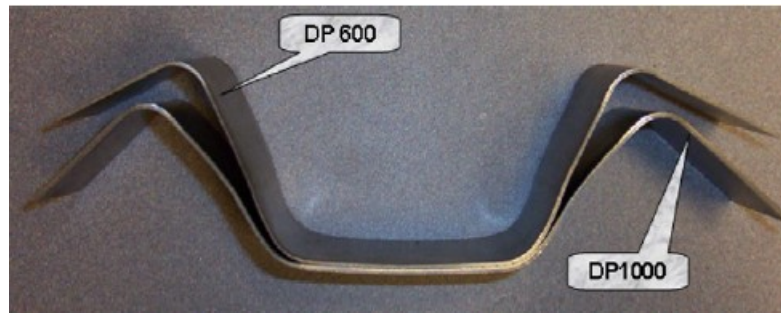
Figure 2.4. Experimental test results of DP 600 and DP 1000 of the U-drawing test (Koc and Chen, 2007). Both materials have been formed using the same process.
