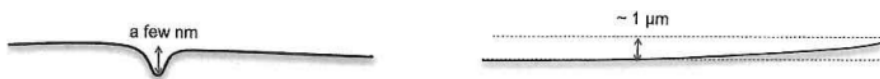
Figure 2.6: Deflectometric sensitivity: (a) Local accuracy can reach down to a few nm. (b) Global accuracy is usually several orders of magnitude worse. [FKR + 12]
