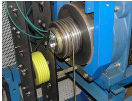
Figure 6.5: Machine, traction sheave and diverting pulley
