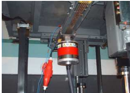
Figure 6.2: Inertial shaker at the bottom of the car
