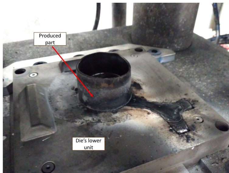
Figure 5.13: The die used in the monitored SSF process, along with the produced part.
