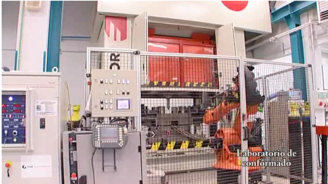
Figure 6.12 Overview of the implemented thixoforging cell.
