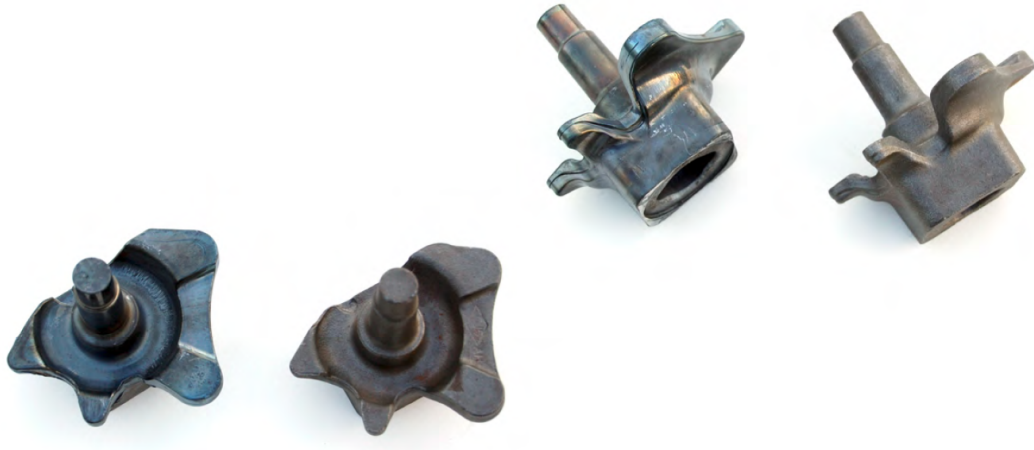
Figure 7.1 Semisolid forged part (left) and hot forged part (right).
