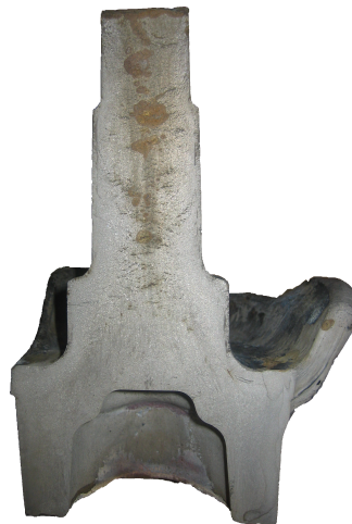
Figure 7.2 Semisolid forged part with defects along the axle.
