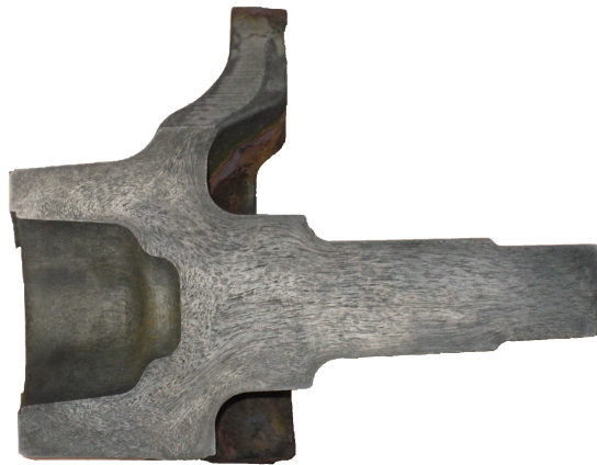
Figure 5.6 Fibre structure of a hot forged spindle.
