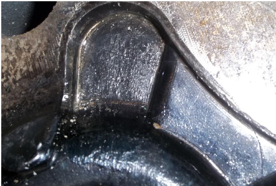
Figure 6.15 Lower die crack.
