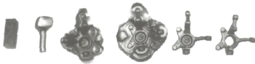
Figure 5.5 Required forming steps for forging a wheel trunk [12].
