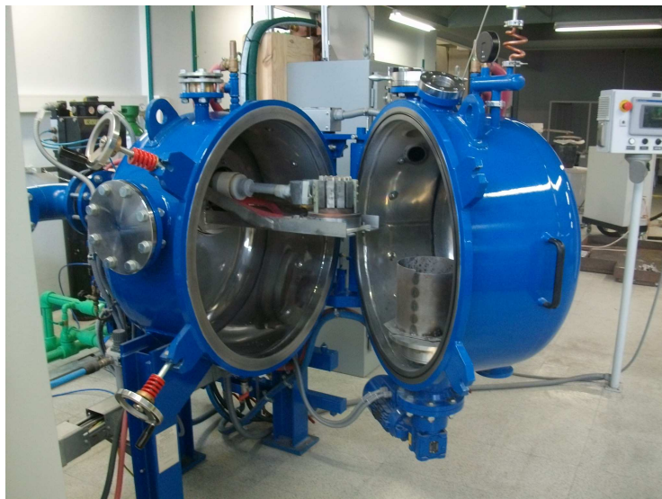
Figure 2.4. A CCIM installation.
