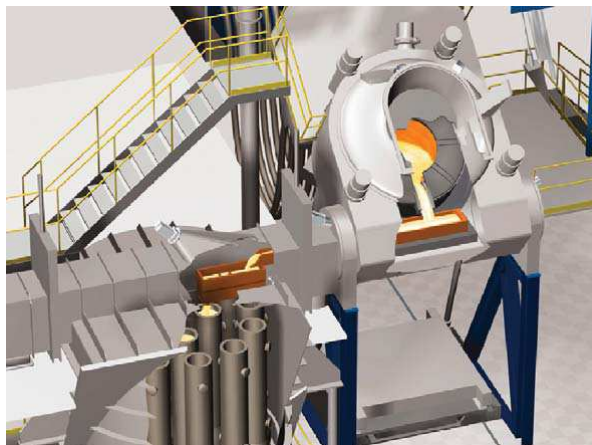
Figure 2.1. Installation of VIM (Zanner 2004).
