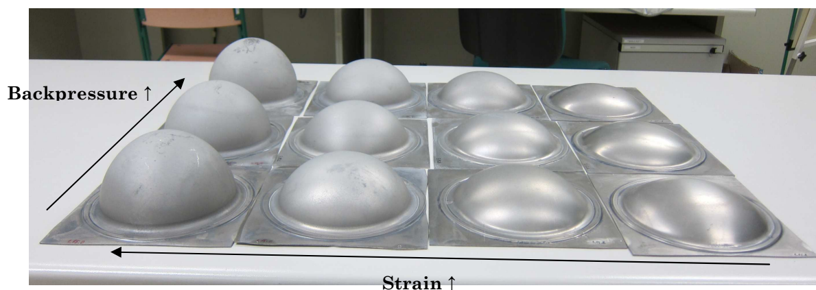
Figure 6.9.: Set of tests made at different backpressure and strain values for 2 \times 10^{-4} \text{ s}^{-1} strain rate.
