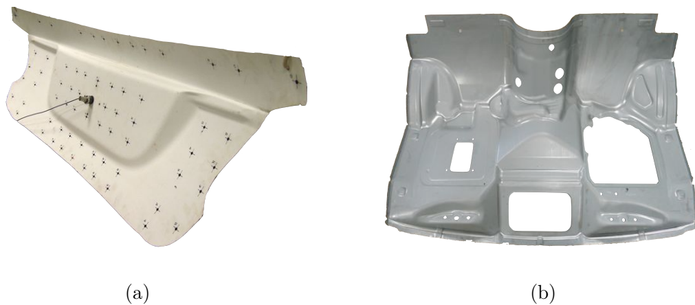
Figure 5.1: (a): Rear door of a car; (b): Panel for isolating the passenger compartment of a van from the engine.
