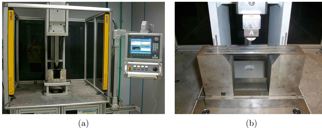
Figure 5.3: (a): General view of the press; (b): Detail of the die and the punch, where three specimens are positioned to be formed at once.
