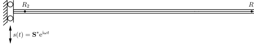
Figure 4.4: Tested 210 mm long CLD cantilever beam subjected to a harmonic transverse base motion s(t) ; R_1 and R_2 response points located 5 mm from the free end and 20 mm from the clamped end, respectively.
