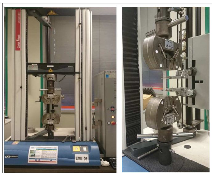
Figure 4 – Machine Used for the Tensile Test
