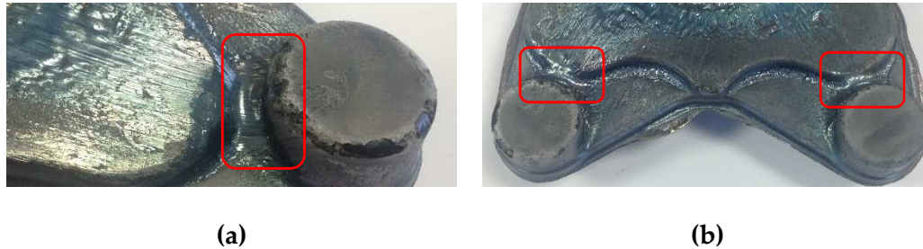
Figure 6.4 – Pictures showing the areas of the component where local wear of dies is appreciated.
