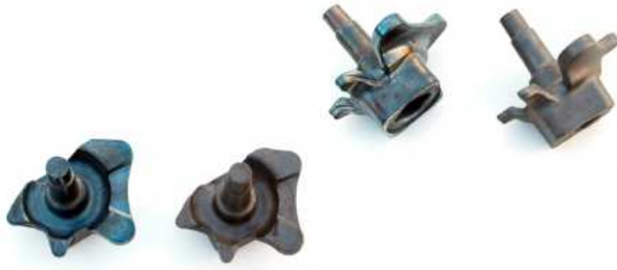
Figure 2.5 – SSF (left) and HF (right) components [46].
