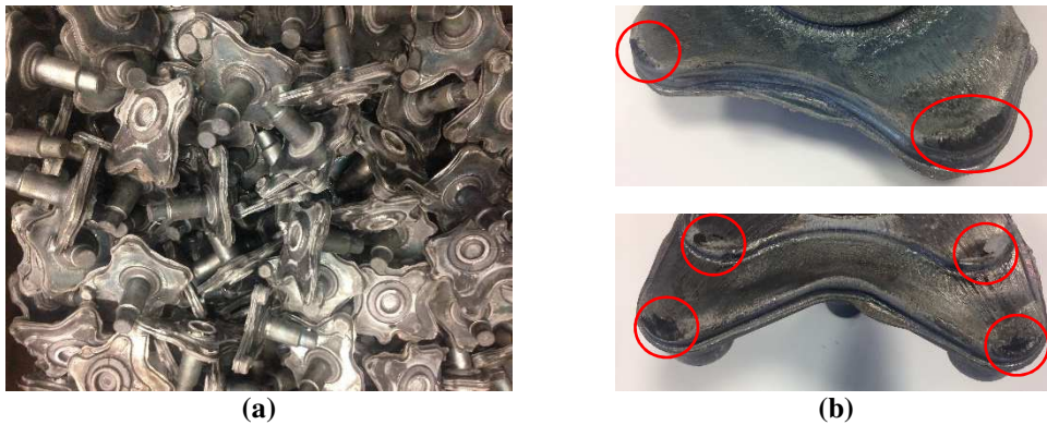
Figure 6.2 – (a) Picture of the fabricated batch and (b) small imperfections due to Ceraspray® entrapment (a).
