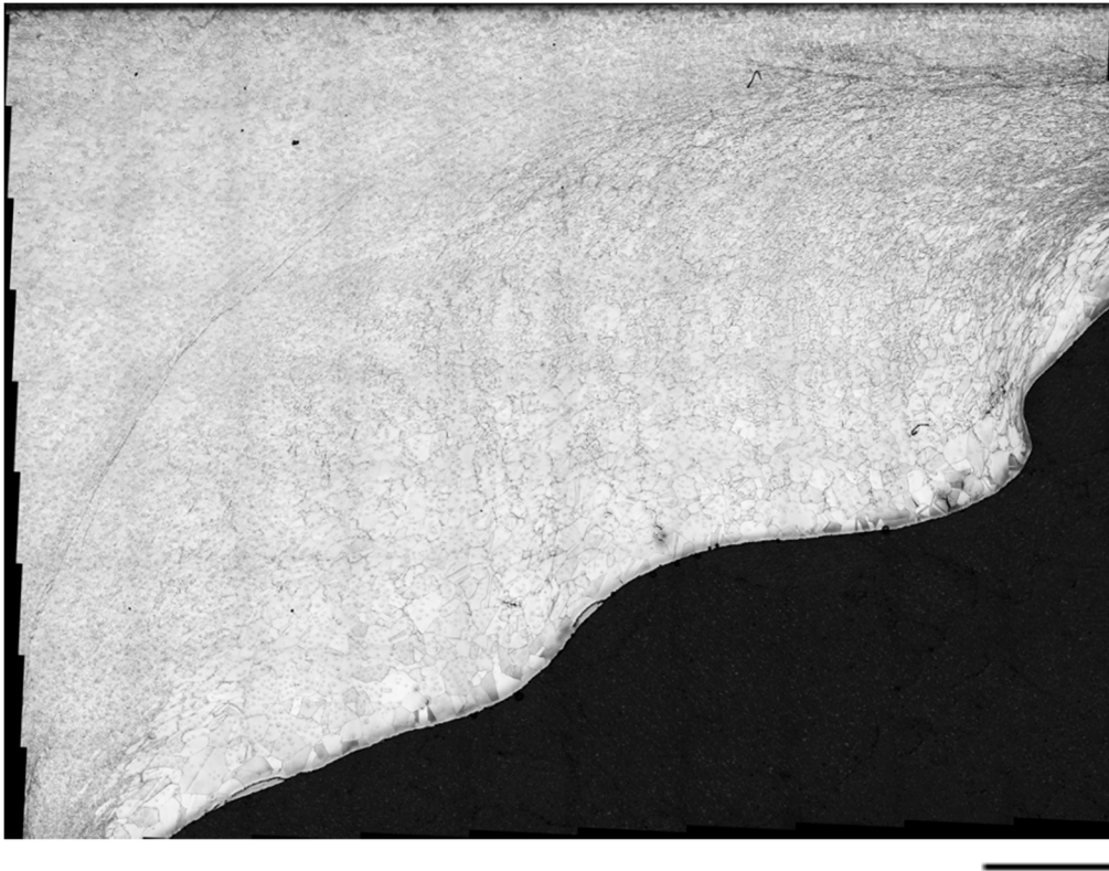
Figure 5.13 – Optical microstructure montage of the corner. Same direction as Figure 5.12. Scale bar: 2mm.
