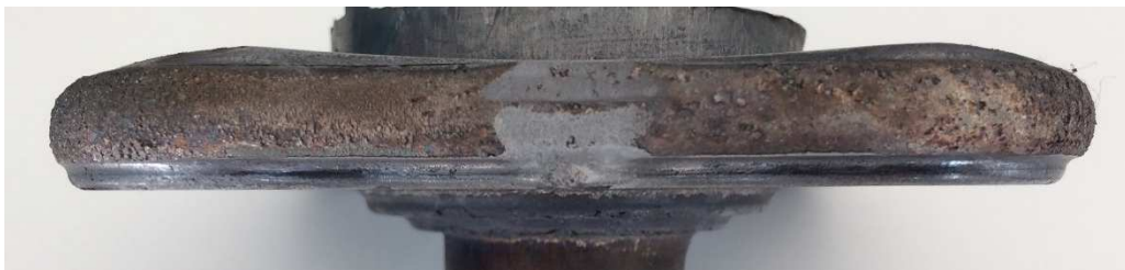
Figure 6.3 – Picture of a component fabricated stopping the process before the cavity was completely filled.
