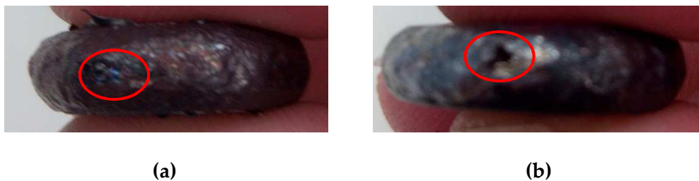
Figure 4.14 – Pictures of deformed samples at 1340^{\circ}\text{C} and (a) 3s^{-1} and (b) 15s^{-1} . The hatched zones show the created cracks.
