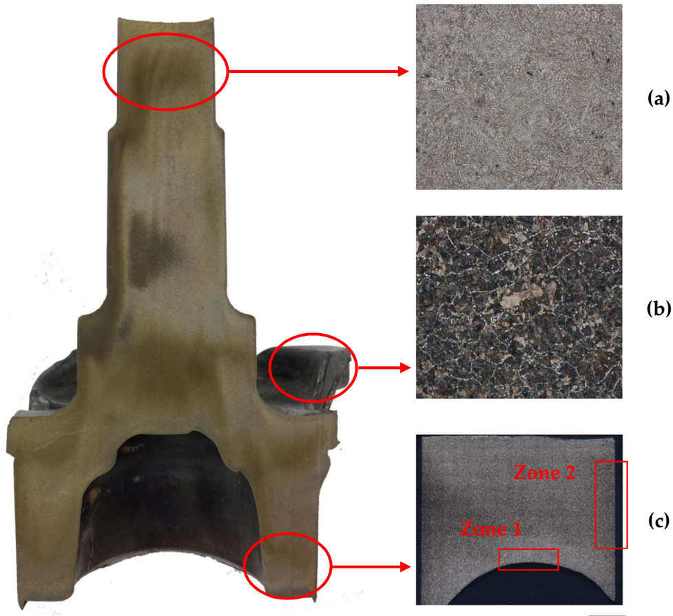
Figure 3.10 – The manufactured SSF component of 44MnSiVS6 cut in half and the microstructures at different positions: (a) axle, (b) middle and (c) bottom. The scale bar means 100 \mu m for (a) and (b) and 5 mm for (c).
