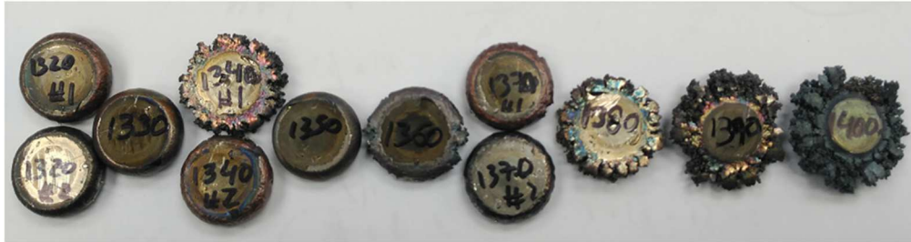
Figure 4.13 – Samples shape after the compression at different temperatures at 3s^{-1} .
