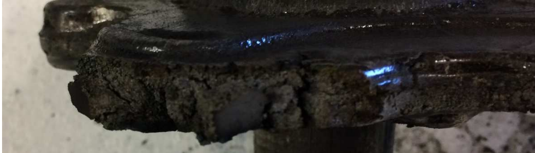
Figure 5.10 – Observed severe grain decohesion in the areas where the flow stopped.
